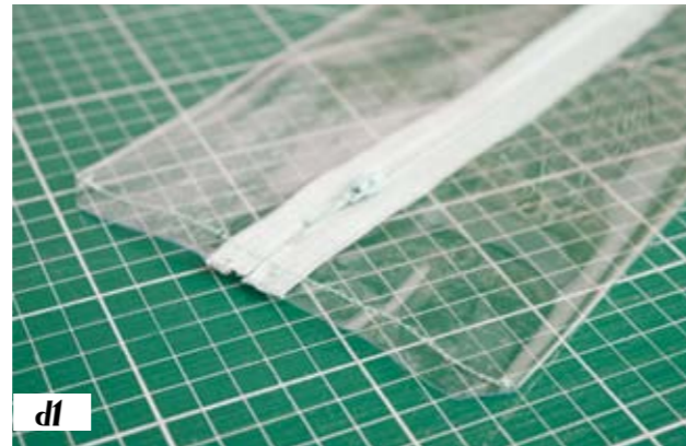
Fig d1 Stitch along the same short edge of the pouch where the zip pull is located. Clip off the corners.
